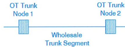
Figure 3-1 Trunk Segment of Leased Line
